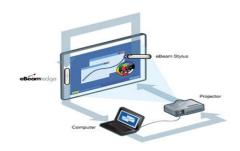
eBeam is an interactive whiteboard system which works with computers and digital projectors. With the help of this technology any standard whiteboard or other surface like wall etc. can be transformed into an "interactive whiteboard". Now we do not have to limit our self to the boundation of surface of whiteboard only but now our screen could be widened as per the need, making it both user and viewer friendly. So it save our money and make session more interactive. [7]
